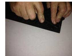
Remember to tensions both sides of the grille cloth while gluing for an even finish.
