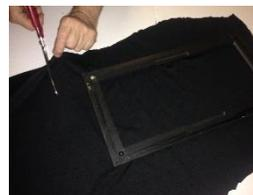
**STEP 5** - Place grille centrally on top of cloth. Using Glue Gun, glue the first corner of the grille
