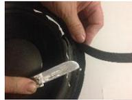
**STEP 3** - Very carefully scrape off old glue from cone. In some instances you may need to peel old glue off or gently rub old glue with an Acetone/alcohol soaked cotton buds.
