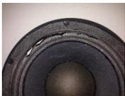
**STEP 2** - Carefully remove gasket/cardboard trims. These parts can be reused (if damaged we do sell replacements). Scrape off old glue from speaker frame with knife, finish off with sandpaper. Gently rub old glue off with an Acetone/alcohol soaked cotton bud
