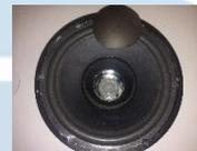
Ensure there is absolutely no contamination in voice coil gap
