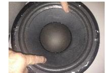
Push surround onto basket until surround stops lifting Allow glue 4-8 hours to set. Remove tissue from under cone if used
